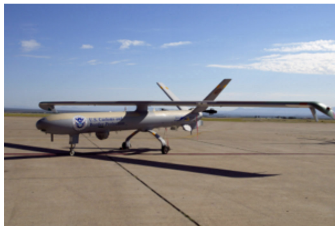
Figure 1. The Hermes 450 unmanned air vehicle, a military system with commercial prospects in civilian applications. (Source: Wikimedia Commons.)
